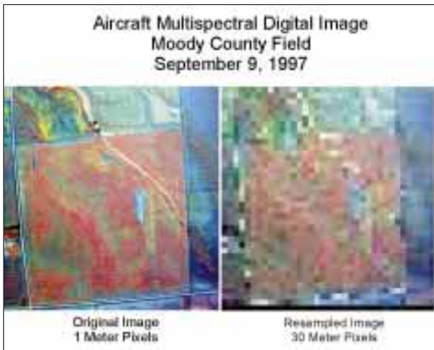
Figure 1. False color imagery of a farm field is represented in two pixel resolutions (1 m versus 30 m pixels). Observable differences in detail between the scenes are obvious from individual trees to drainage definition. Similarities between scenes are seen in the crop vigor (strength of red colors) and northwest-southeast orientation of coloration differences.
